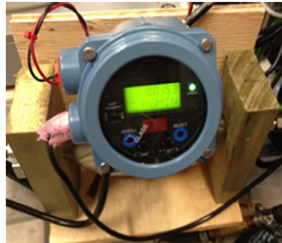
Fig. 5. Refrigerant mass flow meter.
