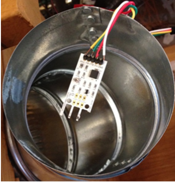
Fig. 7. Air temperature & velocity sensors.
